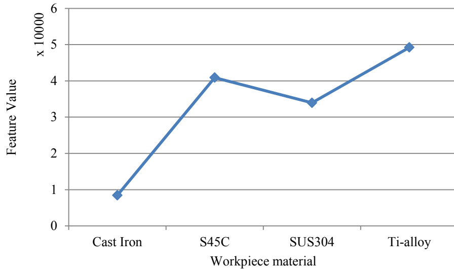
Figure 4-9 The relation between the workpiece material and the geometry feature
