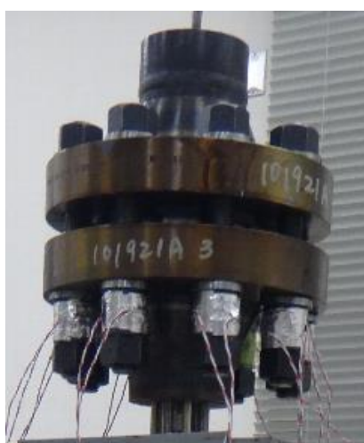
(a) Photo of the bolted pipe flange connection (3B-RTJ)
