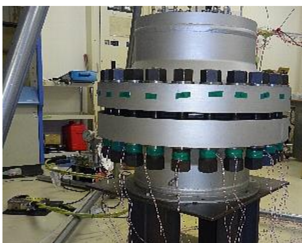
(b) Photo of the bolted pipe flange connection (20B-RTJ)
