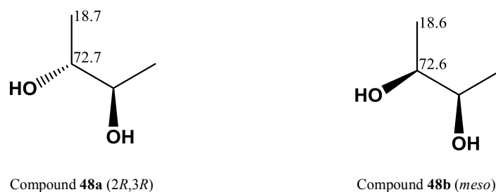
Fig. 19 ^{13}\text{C} NMR data for ( 2R, 3R )- and meso -2,3-butanediol (Compound 48a and 48b )
