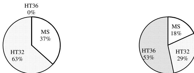
Fig. 2.7 Use ratio of material grades (min. cost of case C). Fig. 2.8 Use ratio of material grades (min. weight of case C).
