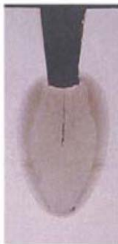
Fig. 2.9 Picture of solidification cracking in the centerline related to a pear-shaped bead [21].
