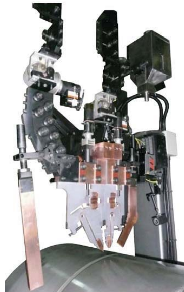
(b) Tandem twin wire SAW welding head and ancillary equipment [43].
