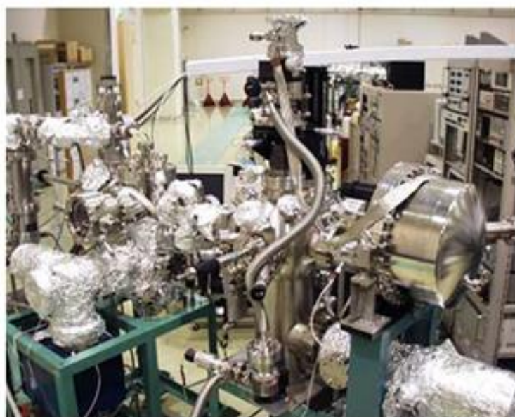
Figure 4.7: BL-7 experimental system. PES spectrometer is equipped with a He cryostat for low temperature experiment. The sample preparation chamber has components of sample cleaning for bulk or surface experiments.
