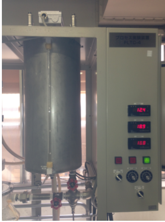
Figure 2.9: Level and temperature-control system.
