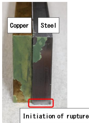
Fig. 3.17 Photograph of ruptured interfaces ( scarf angle is 60°, left adherend is copper, right adherend is steel in the case where the adhesive length is held constant)
