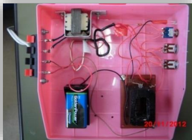
Figure 72. Example of an actual low-cost colorimeter
