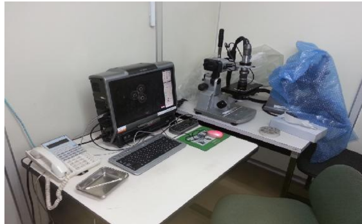
Figure 2.10 The digital microscope
