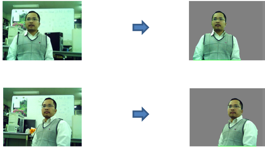
Figure 5-8. Segmentation on stereo video captured by Minoru 3D webcam
