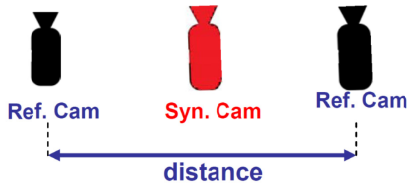
Figure 4-17. Varying the distance between the two reference cameras.
