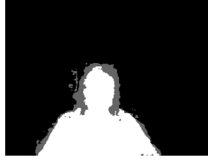
Figure 5-5. Tri-map (black color: background region; white color: foreground region; grey color: uncertainly region).
