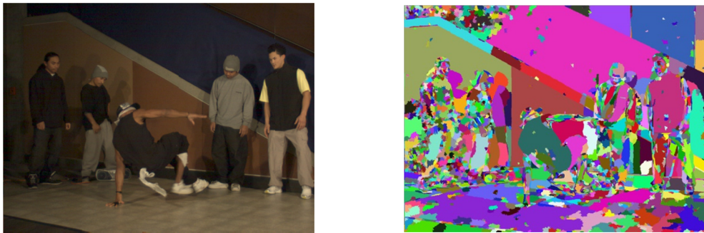
Figure 3-16. Original “Break-dancers” image (on the left) and the corresponding segmented image using mean shift segmentation algorithm (on the right).
