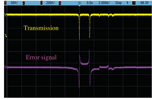
Fig. 12. The transmission and the error signal for the feedback system utilizing the polarization property of the 3D 4-mirror cavity.
