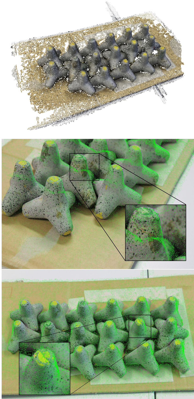
FIGURE 2.15: Estimation results. (top) 3D point cloud. (middle and bottom) Projection of the 3D point cloud with estimated camera poses onto image 26 and 27.
