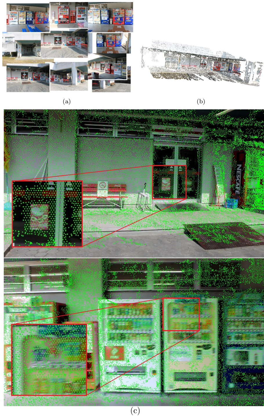
FIGURE 2.16: Estimation results for the outdoor scene. (a) Some training images. (b) Reconstructed 3D point cloud. (c) Two snapshots of query videos with 3D points superimposed.
