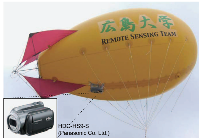
Fig. 2 Picture of the digital video camera and balloon system used in this study.
