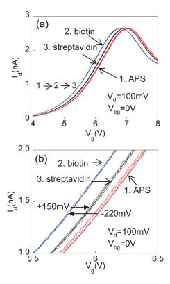
FIG. 2. (Color online) Drain current  $(I_d)$  vs. gate voltage  $(V_g)$  characteristics of SET with multiple islands for biotin-streptavidin binding at room temperature. Drain-source voltage  $(V_d)$  was fixed at  $100\,\mathrm{mV}$ . Back-gate voltage  $(V_{bg})$  was fixed at  $0\,\mathrm{V}$ . The results were for  $10\,\mathrm{-}\mu\mathrm{g/ml}$  streptavidin. (b) Curves in  $V_g$  region from 5.5 to 6.5 V for (a).
