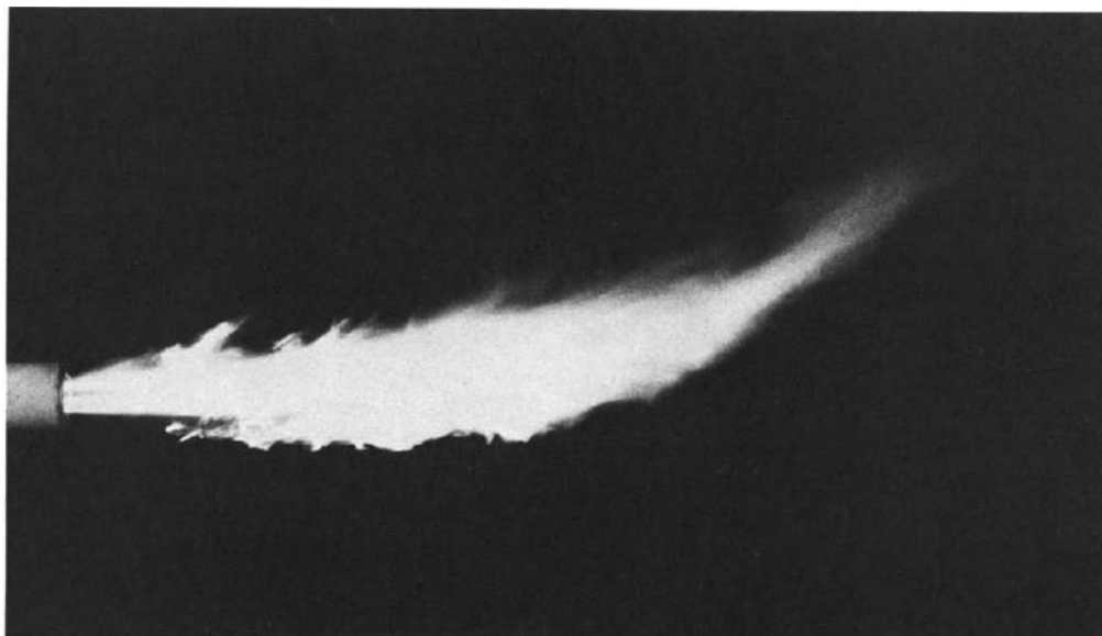
Fig. 1.5 Oxy-methane flame; \Phi = 1 , 190kW [29].
