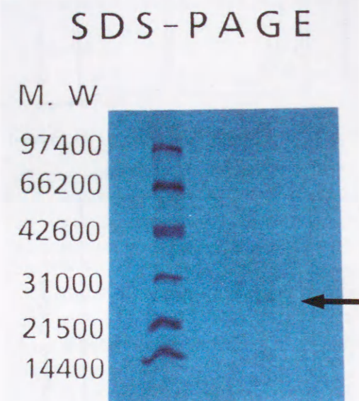
Fig. 4. Molecular weight estimation of urine TGF- \beta by SDS-PAGE. Sample was applied to TEF-CO-GEL SDS-PAGE mini (1 hr, 25 mA) and stained by Cumasie Blue. SDS-PAGE Molecular weight Standards-Low: Rabbit muscle phosphorylase b (97400), Bovine serum albumin (66200), Hen-egg white ovalbumin (42600), Bovine carbonic anhydrase (31000), Soybean trypsin inhibitor (21500), Hen-egg white lysozyme (14400). Single band meaned TGR- \beta appeared in M. W. 25,000 point ( \leftarrow ).
