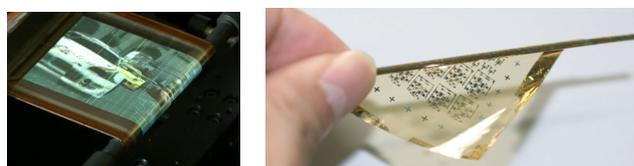
**Figure 1.1.2.** (a) A rollable display demonstrated by Sony in 2009. (b) An ultra-flexible integrated circuit reported by Sekitani *et al.* in 2010.
