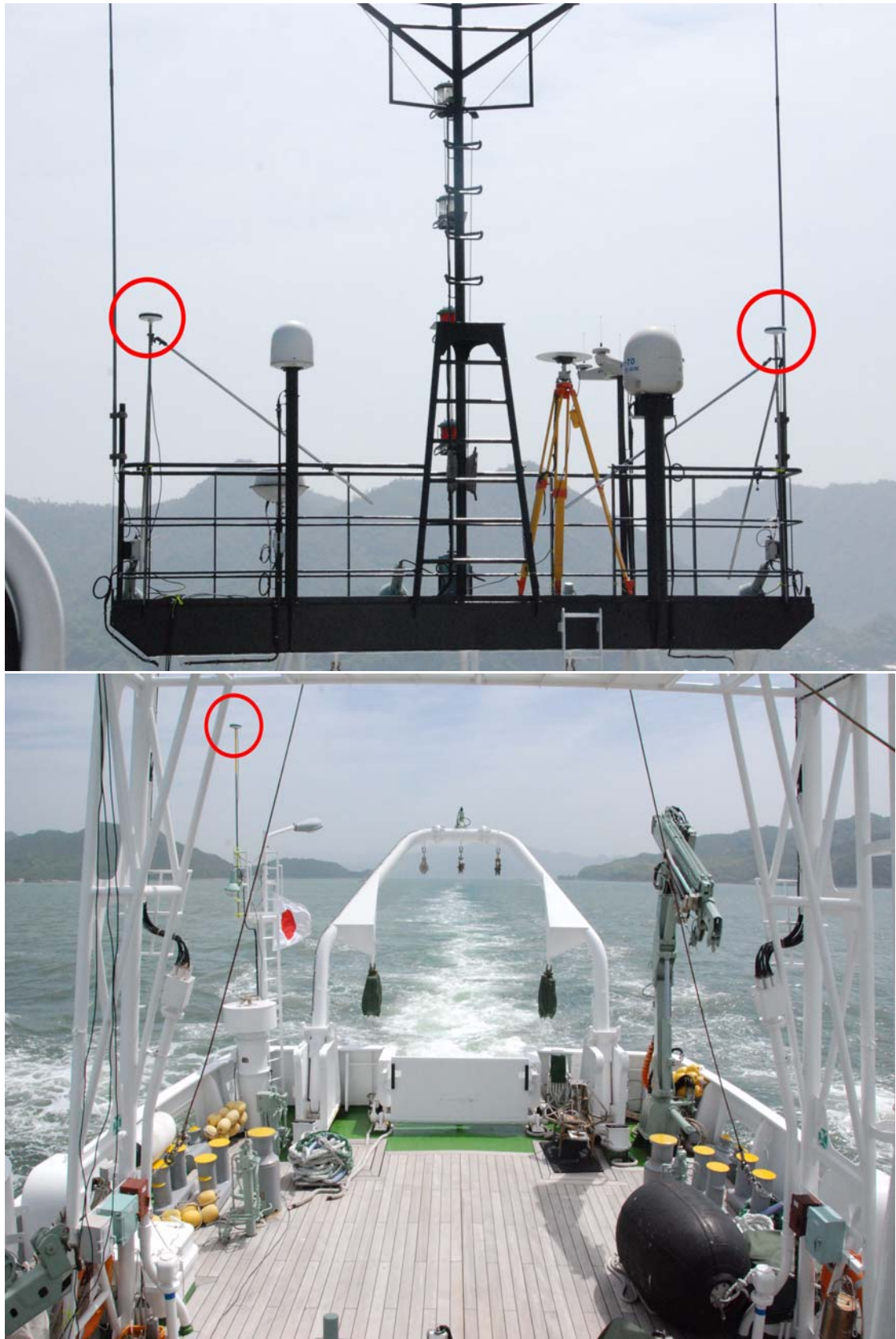
Fig. 4.2: Settings of GPS antennas on “Toyoshio-Maru”
