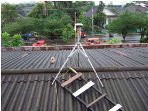
(a) GPS antenna on the roof
