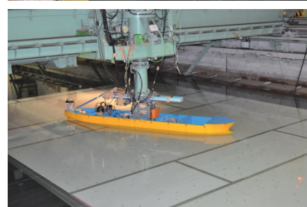
Figure: Experiment in shallow water (Hiroshima University towing tank)
