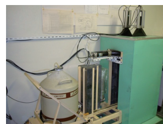
Low-level Ge spectrometer
