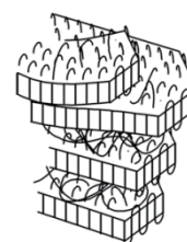
Crystalline-amorphous stacked layers in crystalline polymers
