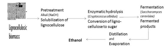
Figure 5. Production of ethanol by degaradation and bioconversion of bagasse of pulp and paper mill effluent using cellulosic hydrolysis by *Cryptococcus albidus* and *Saccharomyces cerevisiae* (Thakur, 2009).
