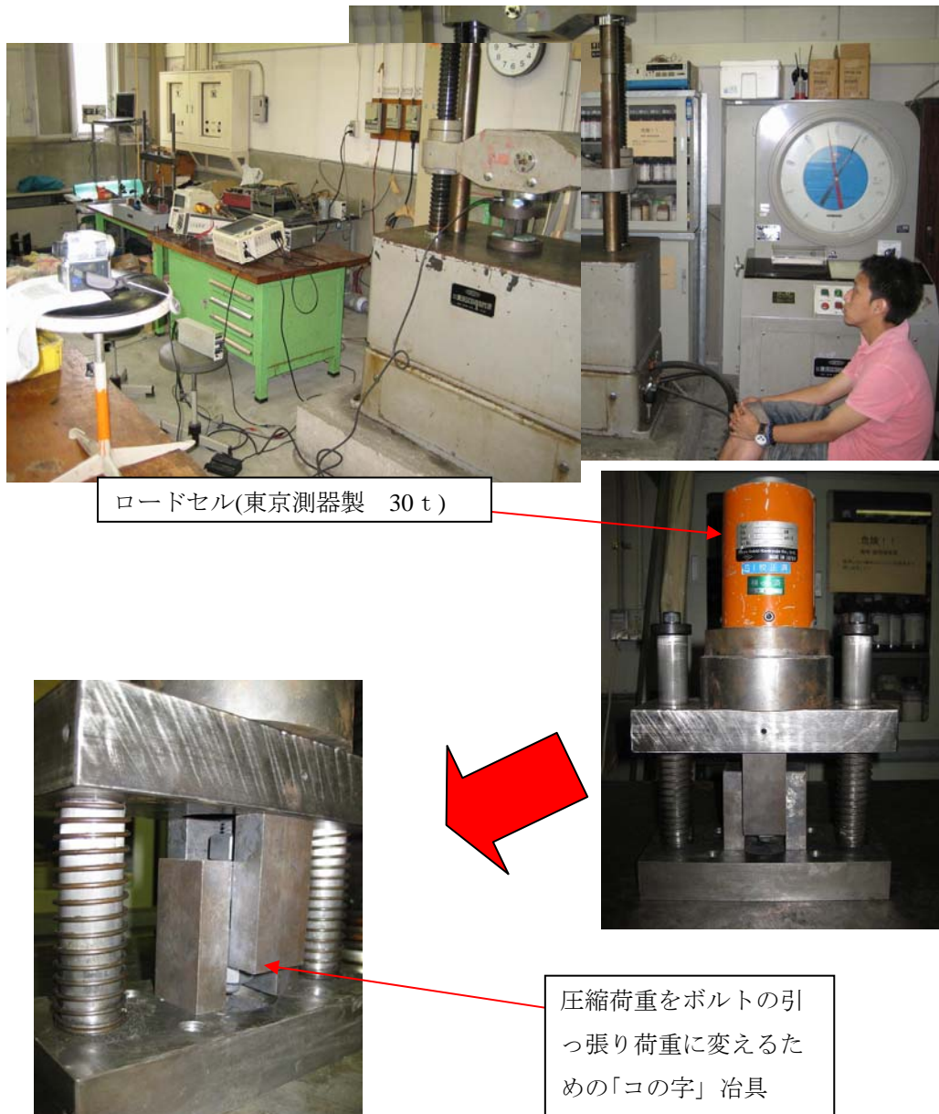
Fig. 6.3.7 Schematic of experimental apparatus for measuring rupture loads
