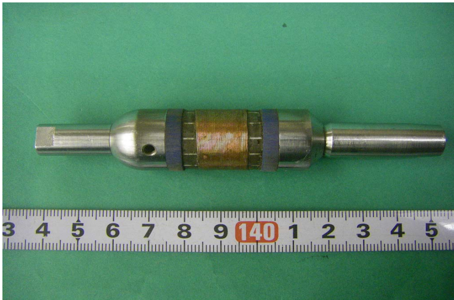
Fig.3.3.1 Appearance of axial-shear EMAT
