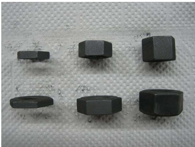
Fig.6.3.6 The photograph of corrosion of the nuts
