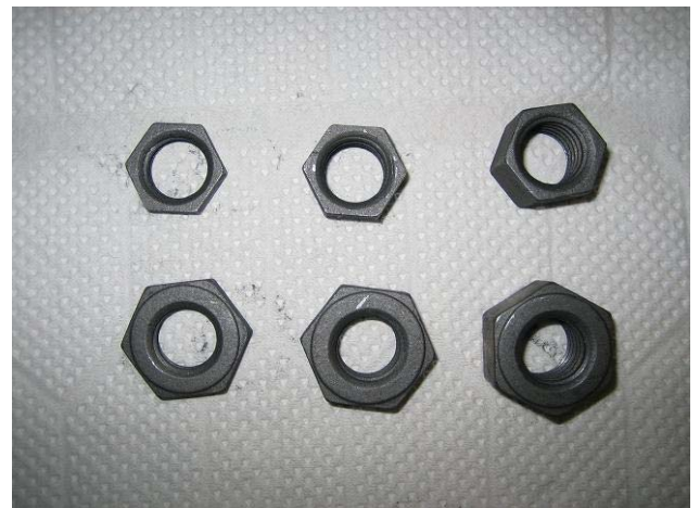
Fig.6.3.6 The photograph of corrosion of the nuts
