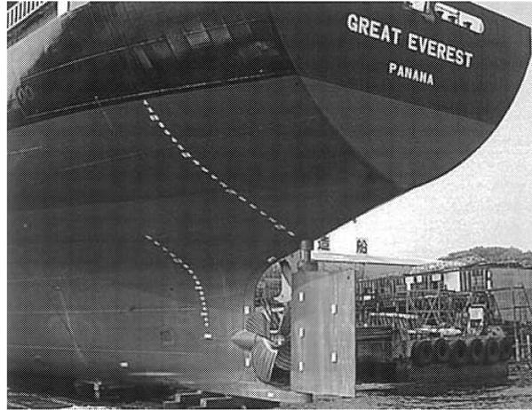
Fig. 6.1: Example of a rudder installed at the stern [40]
