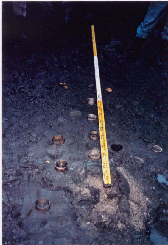
写真-2. 3 沖積粘性土の試料採取 (c)
