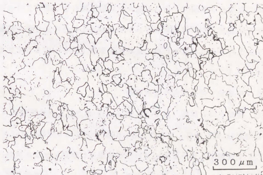
Fig.8-11 Microstructure of T specimen, which was rolled to 2mm thickness after isothermally upset and followed by annealing at 1273K.
