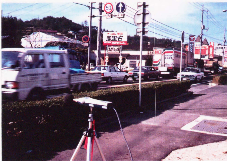
Fig.2.4.7 Actual scene of road traffic noise measurements using the proposed on-line measurement system.
