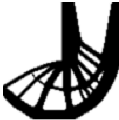
Figure 10: Optimal configurations of the reverse L example
