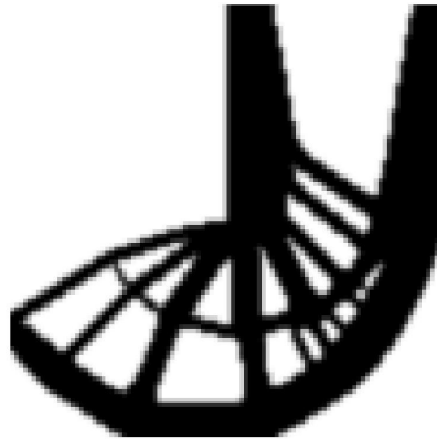
Figure 14: Optimal configurations of the reverse L example obtained by solving the double loop optimization problem
