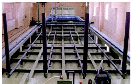
Fig.A-5 Air bubble extractor for high speed flow
