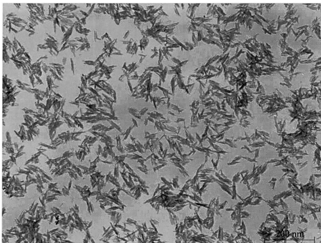
Fig. 1.4 Silicone-coated nano-sized acicular hematite particles.
