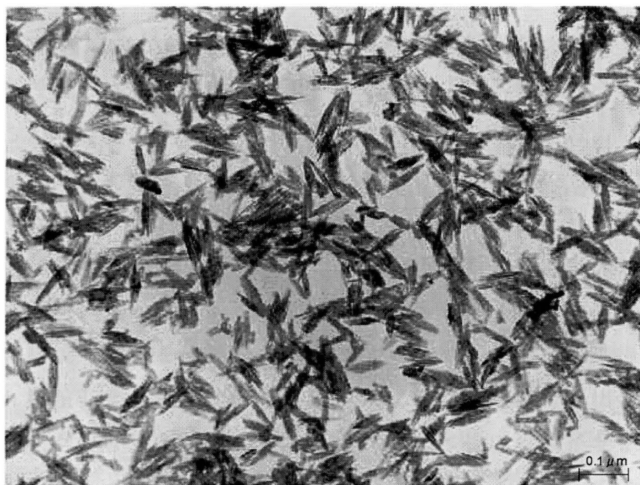
Fig. 6.6 TEM picture of acicular hematite particles at S_{\text{BET}}/S_{\text{TEM}}=1.77 .
