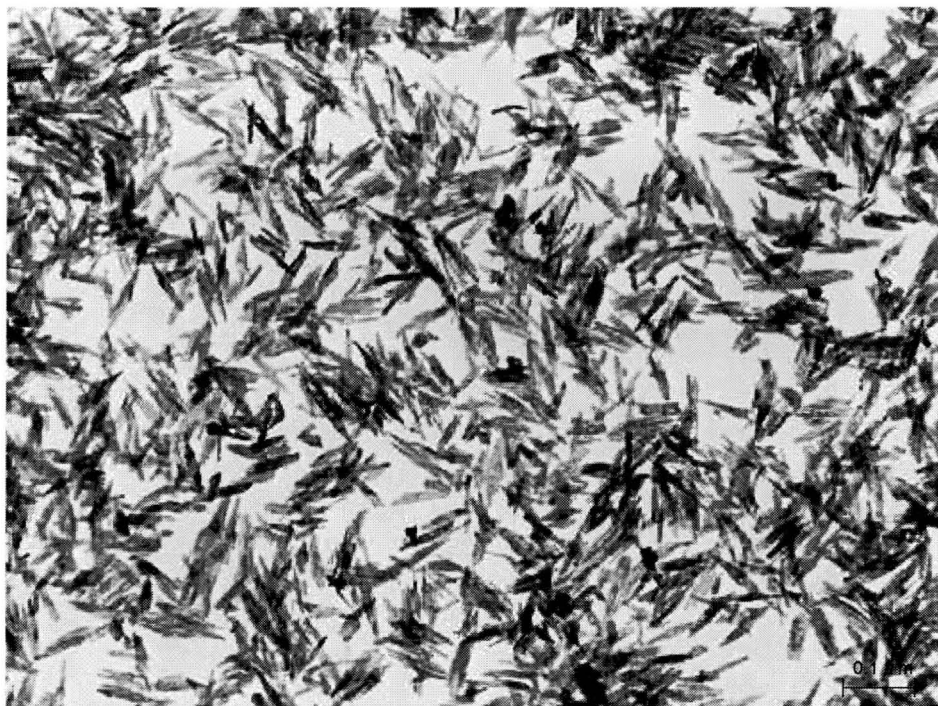
Fig. 6.5 TEM picture of acicular hematite particles at S_{\text{BET}}/S_{\text{TEM}}=1.24 .
