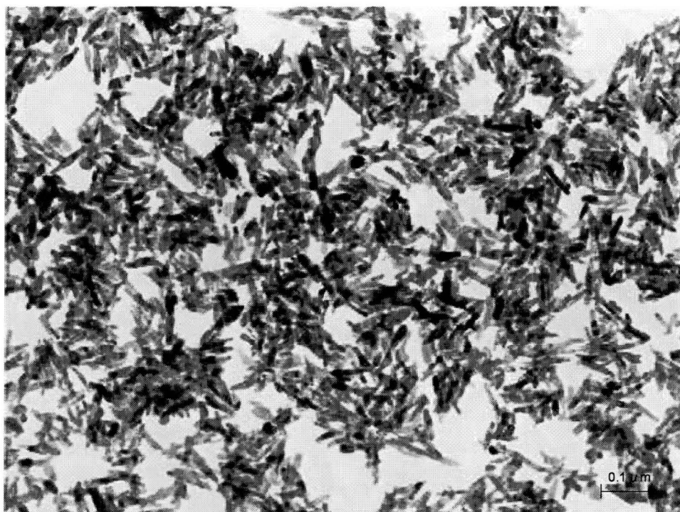
Fig. 6.7 TEM picture of acicular hematite particles at S_{\text{BET}}/S_{\text{TEM}}=0.74 .
