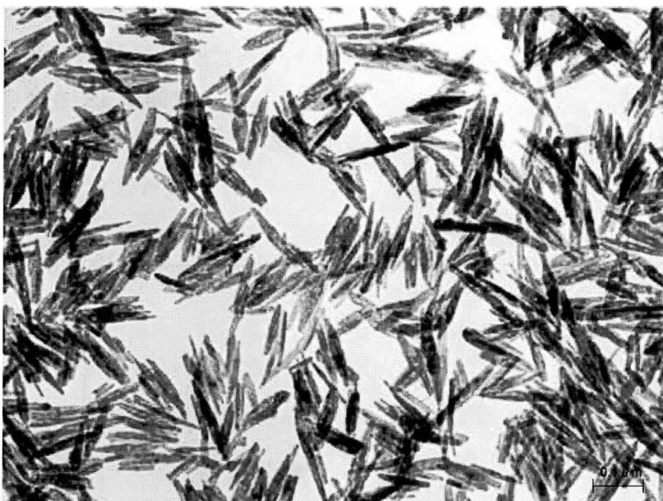
Fig. 6.8 TEM picture of acicular hematite particles whose length was 152nm.
