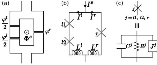
Fig. 1. (a) Schematic diagram of an asymmetric SQUID with three Josephson junctions. (b) Representation of the equivalent circuit, where the cross denotes a Josephson junction element that is described by the resistively shunted junction model as shown in (c).
