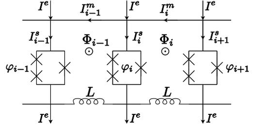
Fig. 2. Equivalent circuit of a SQUID array.
