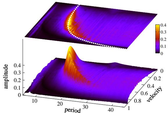
Fig. 4. (Color online). Amplitude of the internal oscillation as a function of the period of external alternating current and the velocity of the bound fluxon pair. The (white) dotted line denotes the relation of the relativistic time dilation.
