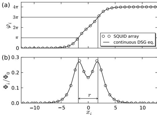
Fig. 3. (a) Phase profile for a fluxon pair when  $d = 0.8$ ,  $\zeta = 4$ , and  $N = 32$ . (b) Magnetic flux through the mesh.
