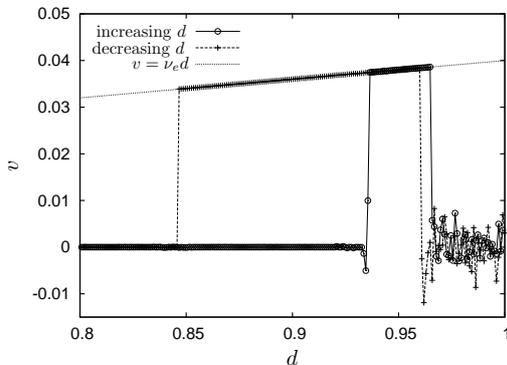
Fig. 5. Mesh size dependence of the average velocity of the fluxon pair.
