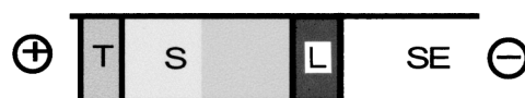
Fig. 1 On-line preconcentration methods for CZE SE: Supporting electrolyte(back ground electrolyte); S: Sample cations; L: Leading electrolyte; T: Terminating electrolyte
