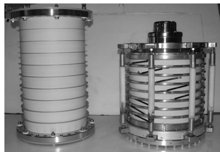
FIG. 1. Segmented ceramic insulators for the 250-kV JAERI FEL gun (right) and the 500-kV ERL gun (left). The guard-ring electrodes are not installed at the 500-kV insulator.
