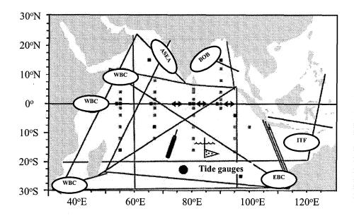
Figure 5: The in situ components of the IndOOS, with moored buoys network, Argo floats, XBT lines, surface drifters and sea level gauges. Source: Meyers and Boscolo 2006
