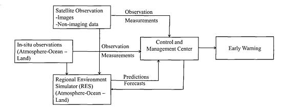
Figure 4: Schematic diagram of the multi-weather hazard early warning system.
