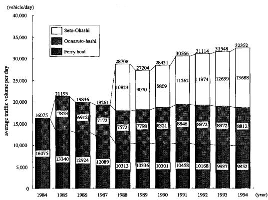
Figure 2 The amount of car traffic between Honsyuu and Shikoku (a quatation from reference 2)
