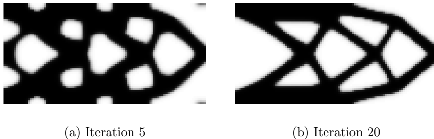
Figure 9: Optimal configurations of the cantilever example on a rougher 100 \times 50 mesh at iterations 5 and 20
