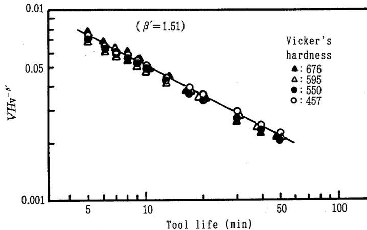
Figure 10. The related line for determining tool-life exponent and Taylor constant in Equation 4, when the value  $\beta'$  is chosen so that the absolute value of the coefficient correlation shows the highest.
