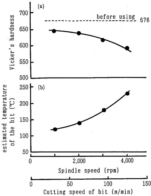
Figure 7. Relationships of spindle speed and cutting speed of bit to Vicker's hardness of cutting edge for non-tempered bit and estimated temperature of the bit at 300 holes.
