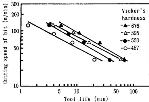
Figure 9. Relationships between tool life and cutting speed of bit with the critical amount of tool wear at  $100 \mu\text{m}$  for four machine bits with different Vicker's hardnesses of cutting edge.
