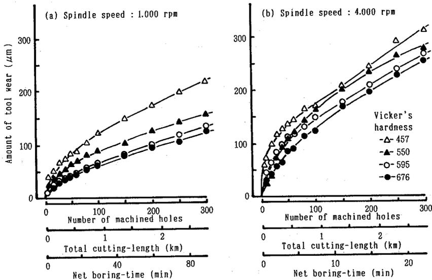
Figure 4. Progressions of tool wear for four machine bits having different Vicker's hardnesses at two spindle speeds.
