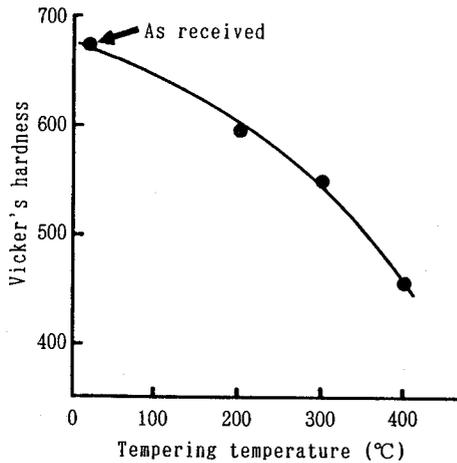
Figure 3. Relationship between tempering temperature and Vicker's hardness of machine bit.
