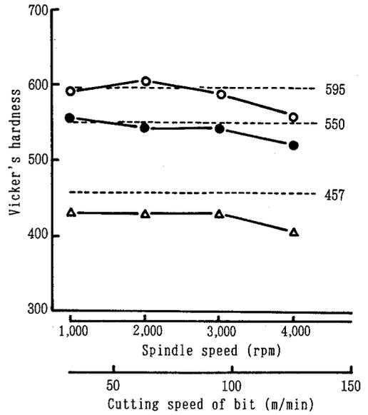
Figure 8. Relationships of spindle speed and cutting speed of bit to Vicker's hardness of cutting edge after boring 300 holes for three kinds of tempered bits.
