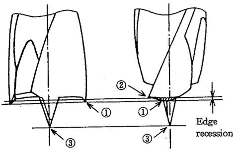
Figure 1. Shape of machine bit used in this test and representation of edge recession.
