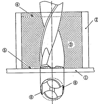
Figure 2. Preparation for measurement of Vicker's hardness of machine bit.
