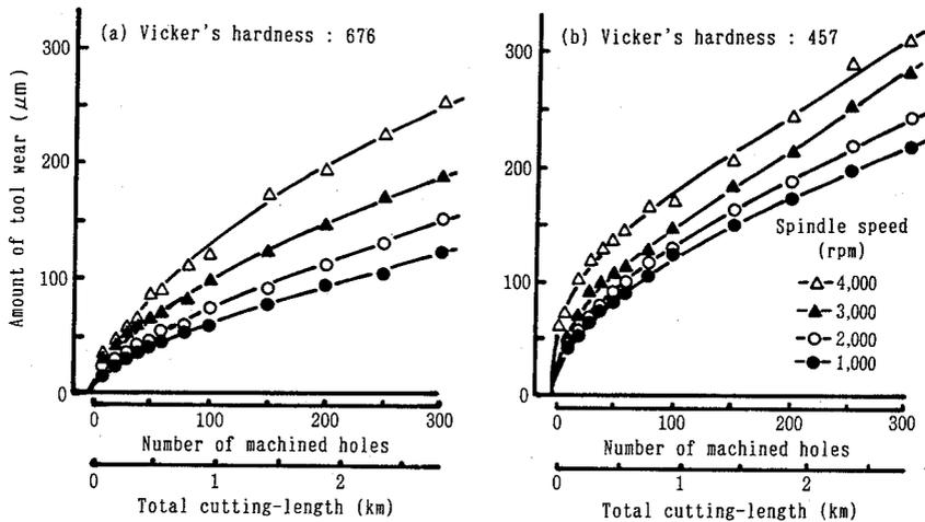
Figure 5. Progressions of tool wear for two machine bits having different Vicker's hardnesses at four spindle speeds.
