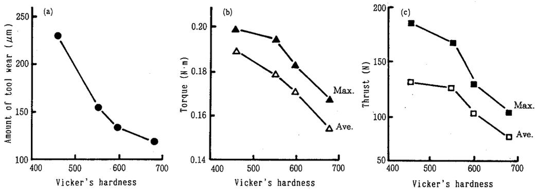
Figure 6. Variations of the amount of tool wear and cutting resistance (torque and thrust) at 300 machined holes with Vicker's hardness of cutting edge of machine bits.
