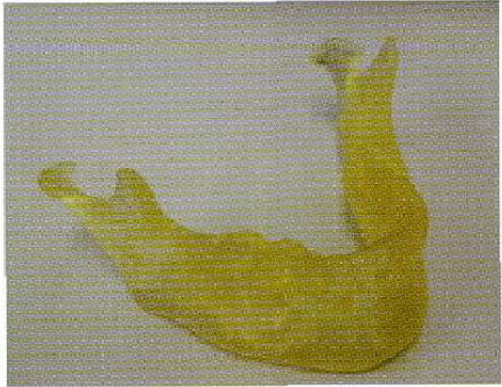
Figure 8: An example of mandible model fabricated using EDEN (OBJET)
