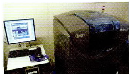
Figure 6: EDEN(OBJET): 3D printing using photosensitive resin
