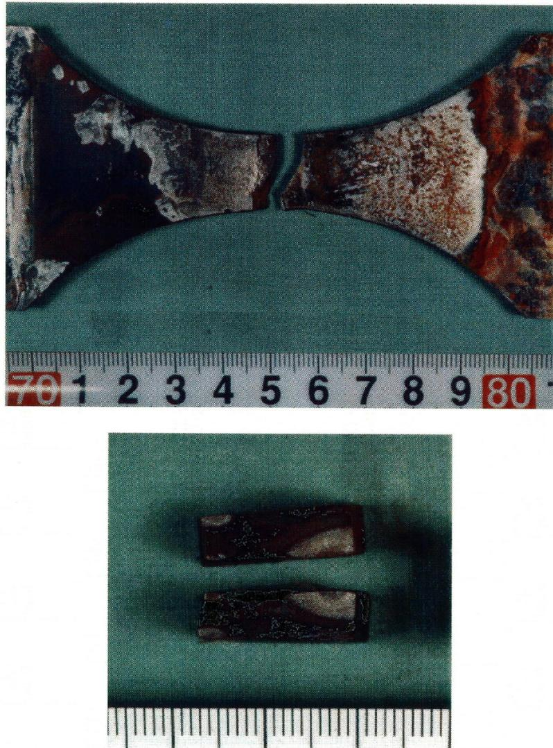
Fig.5.13 Fractured test specimen (In ASW, Boundary section, No.3)
