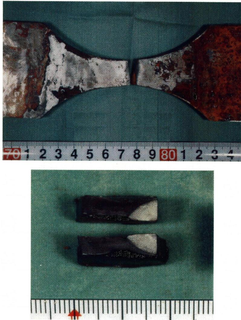
Fig.5.9 Fractured test specimen (In ASW, Surface layer, No.3)
