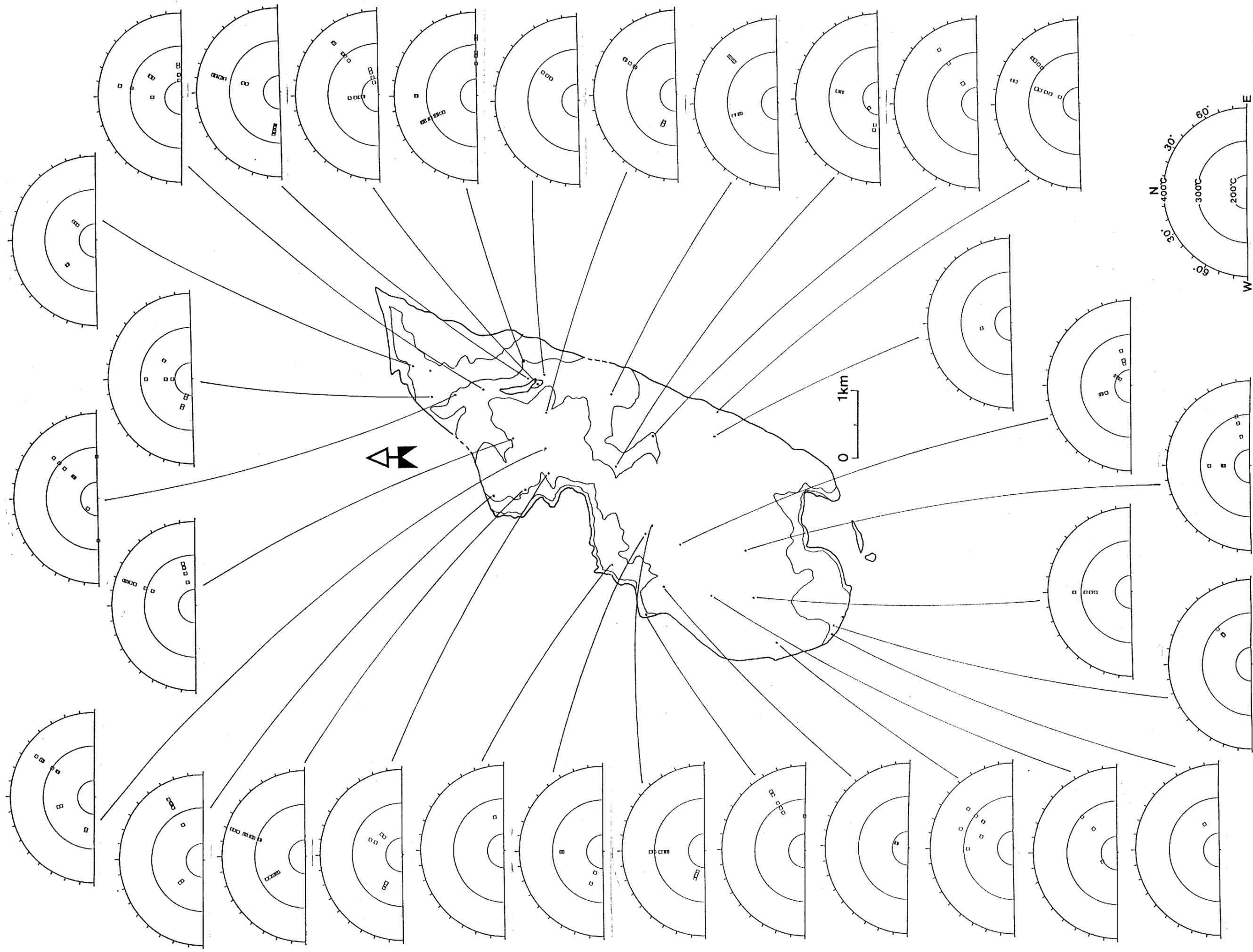
Fig. 61. Spatial variation of the orientation direction of fluid inclusion planes in quartz and their homogenization temperature in the granodiorite and medium-grained granite.
