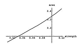
Fig. 3. The nonlinearity of the area of a dipole Rankine ovoid.
