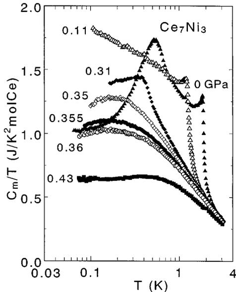
FIG. 4. Magnetic contribution to the specific heat  $C_m/T$  against  $\ln T$  under various pressures.
