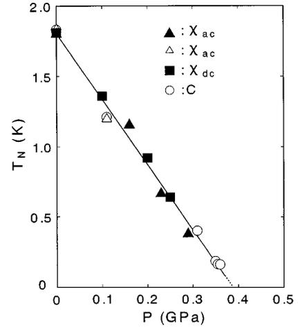
FIG. 5. Pressure dependence of the magnetic transition temperature  $T_N$  for  $\text{Ce}_7\text{Ni}_3$  determined by the measurements of ac [ $\blacktriangle$  (Ref. 12),  $\triangle$ ] and dc susceptibility ( $\blacksquare$ ) and specific heat ( $\circ$ ).
