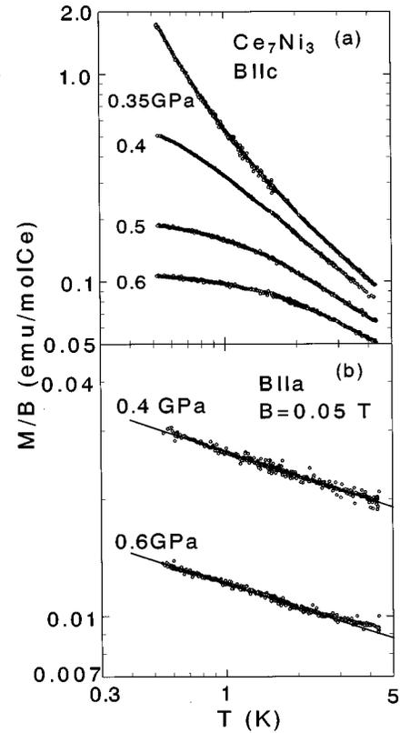
FIG. 6. Magnetic susceptibility  $M/B$  vs  $T$  on a double logarithmic plot at pressures above 0.35 GPa for Ce<sub>7</sub>Ni<sub>3</sub>. Solid lines are fits to a function  $\chi \propto T^{-0.2}$ .
