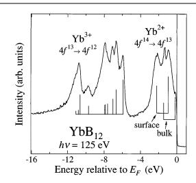
FIG. 2. Valence-band photoemission spectrum of single crystalline YbB<sub>12</sub> ( $h\nu = 125$  eV). Vertical bars for the trivalent part are multiplet structures calculated by Gerken [27].
