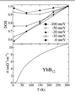
FIG. 4. Top: Spectral DOS of  $YbB_{12}$  at several energy positions as a function of temperature. Bottom: Electrical conductivity of the same sample as a function of temperature.
