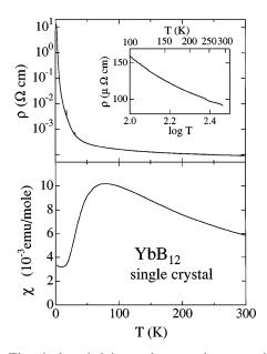
FIG. 1. Electrical resistivity and magnetic susceptibility of the YbB<sub>12</sub> single crystal used in the present work. High-temperature (100 < T < 300 K) resistivity is plotted in the inset.
