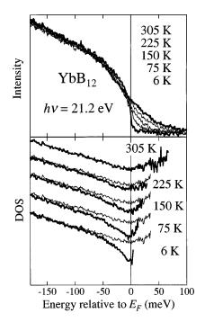
FIG. 3. Top: High-resolution photoemission spectra of YbB<sub>12</sub> near  $E_F$  ( $h\nu = 21.2$  eV). Bottom: Spectral DOS at each temperature (thick curve) together with the DOS at 305 K (thin curve). The bottom line is the zero for the DOS at 6 K and the other densities of states have been offset.
