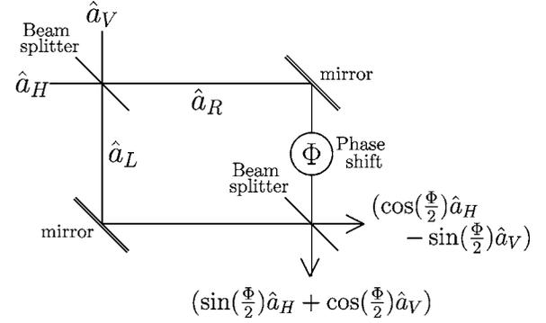
FIG. 3. Illustration of interferometry using the wedge state coherence. By modifying the phases of the  $RL$  modes, the original  $HV$  input is rotated towards the  $PM$  basis. In polarization experiments, the same effect can be achieved by a single half-wave-plate set at  $\theta = \phi/4$  followed by a polarization beam splitter.
