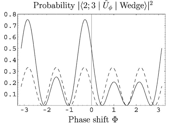
FIG. 4. Probability of finding two photons in the horizontally polarized mode and three photons in the vertically polarized mode as a function of phase shift  $\Phi$  between the circular polarizations for the five-photon wedge state. The dotted line shows the same probability for a corresponding five-photon path-entangled state.
