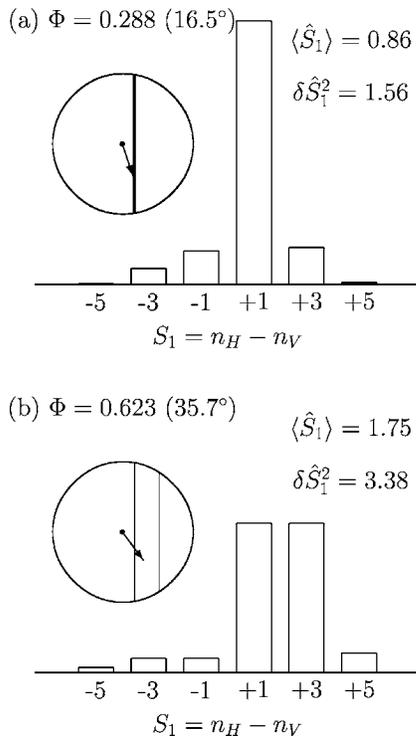
FIG. 5. Measurement probabilities for a five-photon wedge state at phase shifts of (a)  $\Phi=0.288$  and (b)  $\Phi=0.623$ . The corresponding averages and variances of the photon number differences  $\hat{S}_1$  are given in the upper right-hand corners. The sketches to the left of the graphs illustrate the quantized levels with the highest measurement probabilities in the  $S_1$ - $S_2$  plane of the Poincaré sphere. The arrows represent the average Stokes vector of the rotated state.
