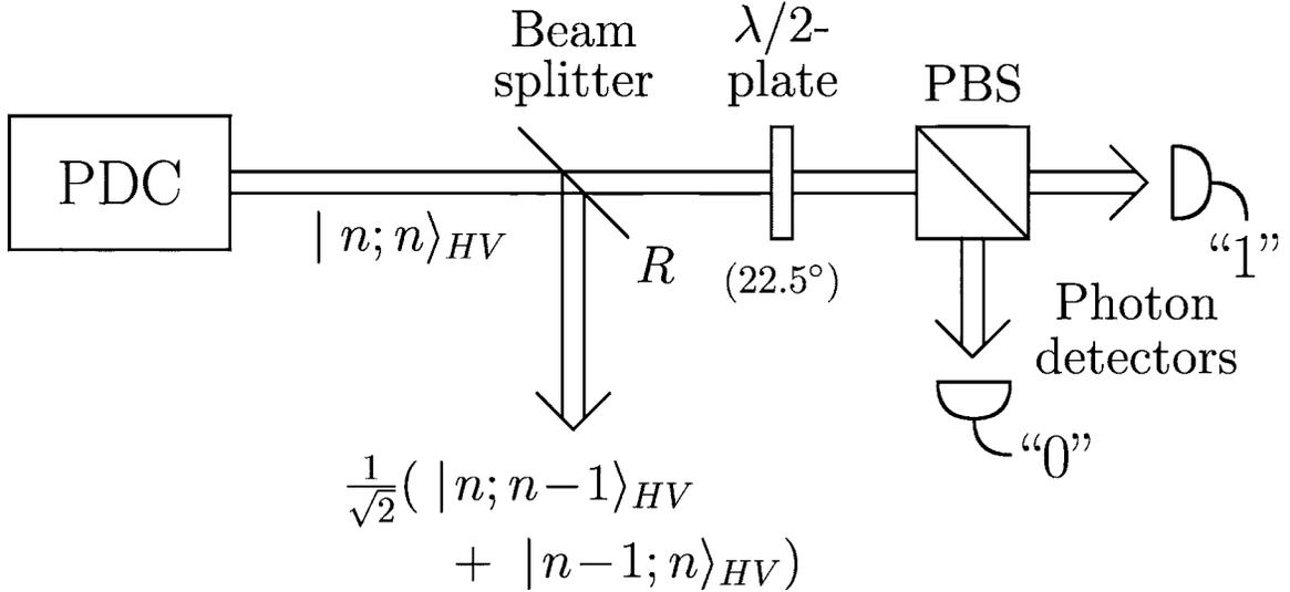
FIG. 1. Sketch of the experimental setup generating the highly-phase-sensitive polarization wedge state. The  $(2n-1)$ -photon state is generated by parametric down-conversion of  $n$ -photon pairs, followed by a reflection of  $2n-1$  photons at a beam splitter of reflectivity  $R$  and detection of the transmitted photon in a diagonally polarized state using a  $\lambda/2$ -plate set at  $22.5^\circ$  and a polarization beam splitter (PBS).
