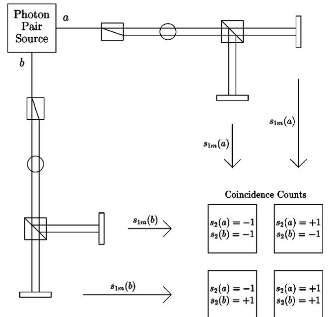
FIG. 3. Schematic representation of the experimental setup for a measurement of polarization correlations on entangled photons. The setup of the branches  $a$  and  $b$  are as shown in Fig. 1. Coincidence counts are registered in one of four channels as illustrated.
