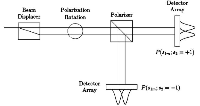
FIG. 1. Schematic representation of the experimental setup for a joint measurement of nonorthogonal polarizations. The beam displacer separates the incoming light into two parallel beams. The polarization is then rotated by an angle of  $\pi/4$  before the light beam is split at the polarizer. The overlapping transversal profile of the beams is illustrated at the detector arrays.
