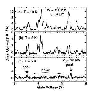
FIG. 5.  $I_d$  vs  $V_g$  characteristics at three different temperatures: (a) T=10 K, (b) T=8 K, (c) T=5 K.  $V_d$  is 10 mV. The nominal wire length and width are 4  $\mu$ m and 120 nm, respectively. The average thickness of the poly-Si wire is  $\sim$ 7 nm.
