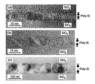
FIG. 3. Cross sectional TEM micrographs of the fabricated poly-Si wires. The average thicknesses of the poly-Si wires are (a)  $\sim$ 7 nm, (b)  $\sim$ 10 nm, and (c)  $\sim$ 82 nm.
