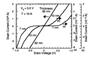
FIG. 2. Drain current  $(I_d)$  vs drain voltage  $(V_d)$  characteristics for three samples with different poly-Si thicknesses. Gate voltage  $V_g$  is 0.0 V. The measurement temperature is 10 K. The nominal length (5  $\mu$ m) and width (100 nm) of the three samples are almost constant. The average thicknesses of the three samples are  $\sim$ 7 nm (from 4 to 9 nm),  $\sim$ 10 nm (from 8 to 12 nm), and  $\sim$ 82 nm (from 80 to 86 nm).
