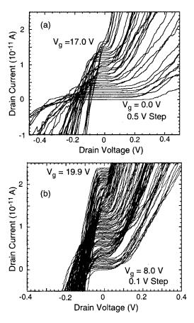
FIG. 4.  $I_d$  vs  $V_d$  characteristics as a function of substrate voltage ( $V_g$ ) at 6 K(a)  $V_g$  from 0.0 to 17.0 V in  $V_g$  steps of 0.5 V. Each curve is offset by 0.5 pA of  $I_d$  for clarity. (b)  $V_g$  from 8.0 to 19.9 V in  $V_g$  steps of 0.1 V. Each curve is offset by 0.2 pA. The nominal wire length and width are 5  $\mu$ m and 170 nm, respectively. The average thickness of the poly-Si wire is ~7 nm.
