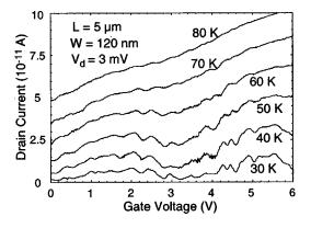
FIG. 8.  $I_d$  vs  $V_g$  characteristics of poly-Si wire at  $V_d$ =3 mV for various temperatures from 30 to 80 K. The conductance oscillations are observed up to about 80 K. The nominal wire length and width are 5  $\mu$ m and 120 nm, respectively. The average thickness of the poly-Si wire is  $\sim$ 7 nm.
