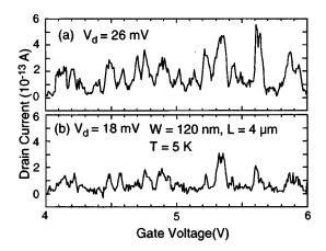
FIG. 6.  $I_d$  vs  $V_g$  characteristics at two different drain voltages: (a)  $V_d=26$  mV and (b)  $V_d=18$  mV. The graph for  $V_d=10$  mV is the same as that shown in Fig. 5(c). The measurement temperature was 5 K. The nominal wire length and width are 4  $\mu$ m and 120 nm, respectively. The average thickness of the poly-Si wire is ~7 nm.
