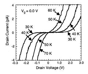
FIG. 7.  $I_d$  vs  $V_d$  characteristics at four different temperatures.  $V_g$  is 0.0 V. The nominal wire length and width are 7  $\mu$ m and 120 nm, respectively. The average thickness of the poly-Si wire is  $\sim$ 7 nm.
