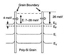
FIG. 10. Proposed energy-band diagram for the smallest island in the poly-Si wire. E is the energy level when one electron is added to the island.
