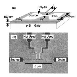
FIG. 1. (a) Schematic diagram of fabricated transistor structure with a narrow, extremely thin poly-Si wire. The average sample thicknesses are  $\sim$ 7,  $\sim$ 10, and  $\sim$ 82 nm. The nominal wire length *L* and the width *W* of the fabricated pattern are 4, 5, and 7  $\mu$ m and 95–2000 nm, respectively. (b) Plan-view SEM of the fabricated poly-Si wire. The wire length and the width are 5  $\mu$ m and 175 nm, respectively.
