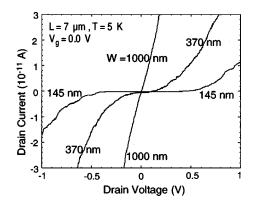
FIG. 11. Wire width dependence of  $I_d$  vs  $V_d$  characteristics at 5 K.  $V_g$  is 0.0 V. The length of the measured wires is constant (7  $\mu$ m). The average thickness of the poly-Si wires is constant (~7 nm).
