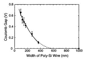
FIG. 12. Wire width dependence of Coulomb gap at 5 K. The length of the measured wires is constant (7  $\mu$ m). The average thickness of the poly-Si wires is constant ( $\sim$ 7 nm).
