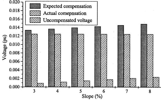
Fig. 11 Available compensation with different slope setting.
