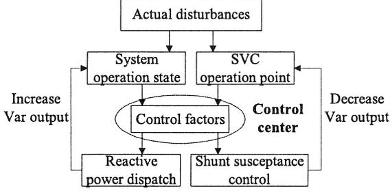
Fig. 5 Schematic design to operation point control.
