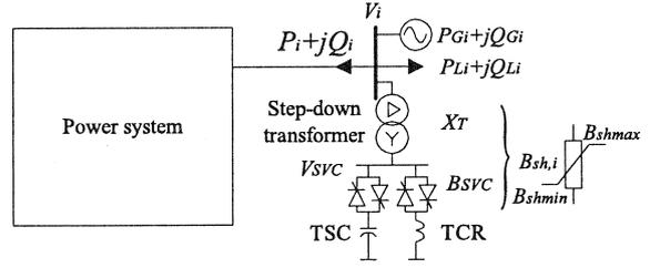
Fig. 2 SVC compensated bus for power flow analysis.
