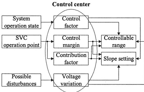
Fig. 6 Schematic design to feasible slope setting.
