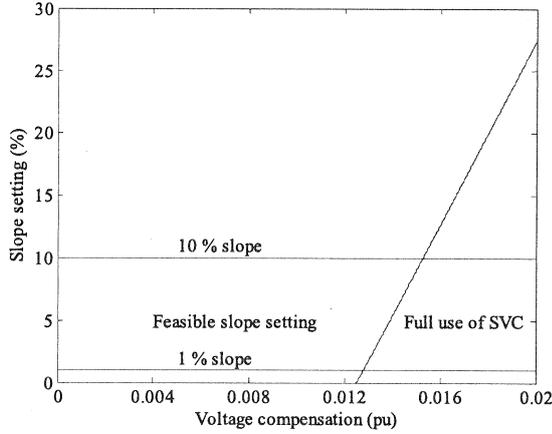
Fig. 12 Slope setting with fixed available control margin.
