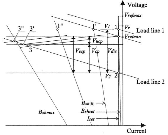
Fig. 4 Steady state V-I characteristic of SVC.
