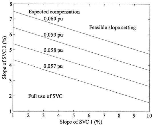
Fig. 13 Slope setting for coordination between two SVCs.
