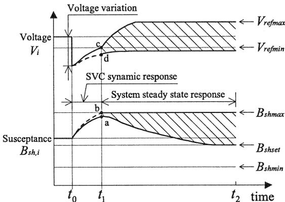
Fig. 1 Post-disturbance reaction of SVC to voltage drop.
