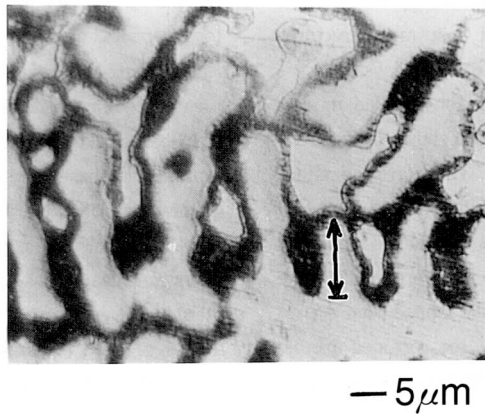
Fig. 8 An example of microstructure in developed Ni-Cu-Mn based alloy when melted in vacuum atmosphere. Arrow shows dendrite arm length indicating the finding of dendrite structures.
