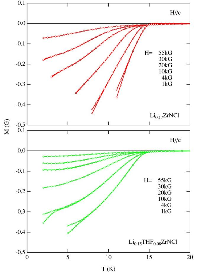
FIG. 8. (Color online) Temperature dependence of the magnetization of (a)  $\text{Li}_{0.17}\text{ZrNCl}$  and (b)  $\text{Li}_{0.15}\text{THF}_{0.08}\text{ZrNCl}$  in external magnetic fields applied parallel to the  $c$  axis. For the plotted data, the quartz ampule background is corrected and the weak-ferromagnetic contribution is subtracted.
