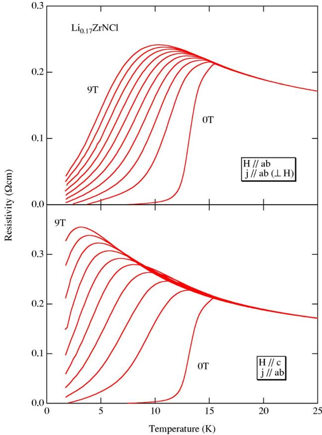
FIG. 11. (Color online) Temperature dependence of the resistivity of  $\text{Li}_{0.17}\text{ZrNCl}$  under external magnetic field for two sets of the field and current directions, measured using a four-probe contact. The applied fields range from 0 to 9 T, in the intervals of 1 T.
