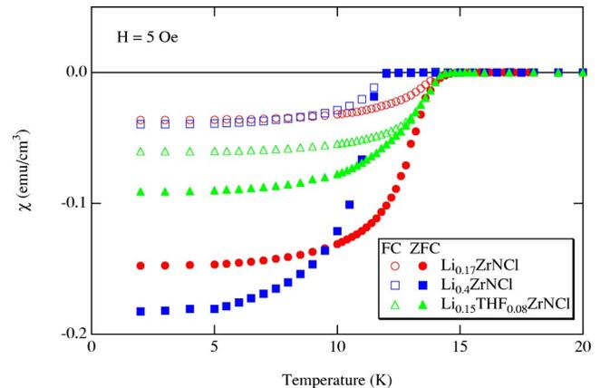
FIG. 2. (Color online) Magnetic susceptibility  $\chi$  vs temperature measured in  $H = 5$  Oe in the field-cooling (FC) and zero-field-cooling (ZFC) procedures in the specimens of intercalated ZrNCl which were used in the  $\mu\text{SR}$  measurements.
