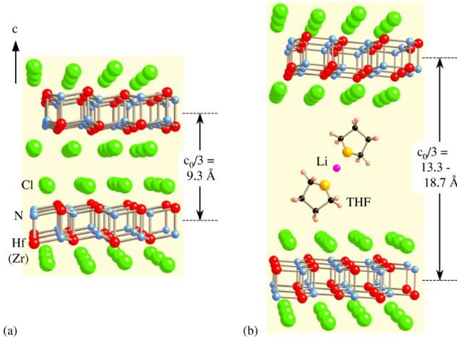
FIG. 1. (Color online) Schematic figures of the crystal structure of Hf(Zr)NCl (a) without intercalation and (b) cointercalated with Li and THF. The stacking unit thickness ( $=c_0/3$ , where  $c_0$  is  $c$ -axis lattice constant) is also shown.
