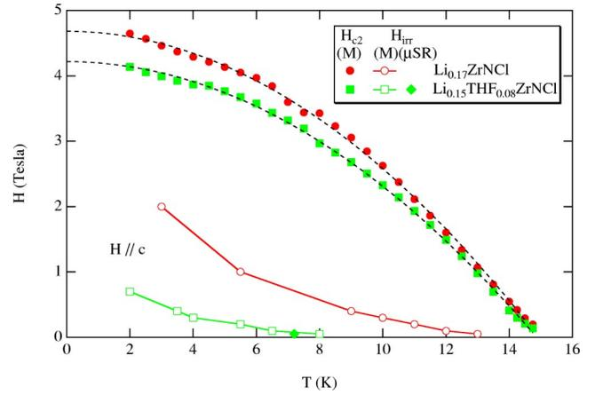
FIG. 10. (Color online) Temperature dependence of the upper critical field  $H_{c2,\parallel c}$  and the irreversibility field  $H_{irr}$  in  $\text{Li}_{0.17}\text{ZrNCl}$  and  $\text{Li}_{0.15}\text{THF}_{0.08}\text{ZrNCl}$ .  $H_{c2,\parallel c}$  was obtained from magnetization measurements (abbreviated as  $M$  in the figure), and  $H_{irr}$  from magnetization and TF- $\mu\text{SR}$  measurements. The broken lines show a fit to the functional form of  $H_{c2}$  given in the text.
