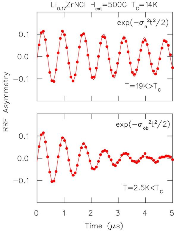
FIG. 4. (Color online) The time spectra of muon asymmetry  $A(t)$  measured in  $\text{Li}_{0.17}\text{ZrNCl}$  at (a)  $T=19\text{ K}$  (above  $T_c$ ) and (b)  $T=2.5\text{ K}$  (well below  $T_c$ ) under the transverse external field of 500 G. The apparent precession frequency in this graph is modified from the actual precession frequency by the use of a rotating reference frame. The solid lines show a fit to Gaussian decay envelope.
