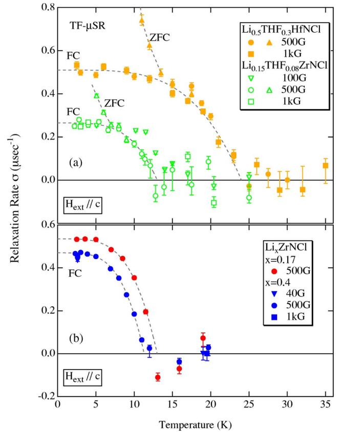
FIG. 5. (Color online) Temperature dependence of the muon spin relaxation rate  $\sigma(T)$  in (a)  $\text{Hf}(\text{Zr})\text{NCl}$  cointercalated with Li atoms and THF, and (b)  $\text{Li}_x\text{ZrNCl}$  without cointercalation. The upper panel (a) shows the results obtained in the field cooling (FC) and zero-field cooling (ZFC) procedures, while the results in the lower panel (b) were obtained in the FC procedure. Dashed lines are guides to the eyes.
