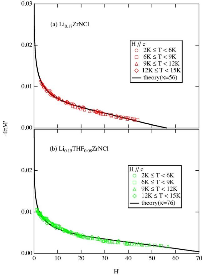
FIG. 9. (Color online) Magnetization as a function of applied field (parallel to the  $c$  axis) in (a)  $\text{Li}_{0.17}\text{ZrNCl}$  and (b)  $\text{Li}_{0.15}\text{THF}_{0.08}\text{ZrNCl}$ , shown in the reduced (dimensionless) units. The solid curves represent a fit to the model of Hao *et al.* (Ref. 30).
