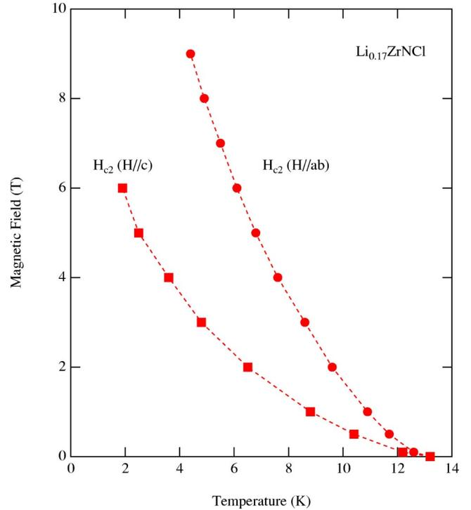
FIG. 12. (Color online) Temperature dependence of the upper critical field  $H_{c2}$  of  $\text{Li}_{0.17}\text{ZrNCl}$ , obtained from magnetoresistance.
