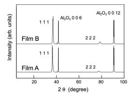
FIG. 1. X-ray diffraction patterns of epitaxial *B*1-MoN films on  $\alpha$ -Al<sub>2</sub>O<sub>3</sub>(001).
