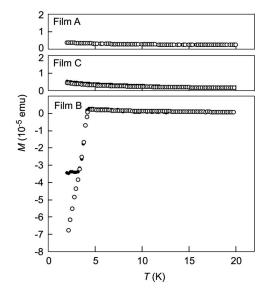
FIG. 2. Temperature dependence of magnetic moment for *B*1-MoN films. Open and solid circles represent zero-field cooling and field cooling, respectively. Magnetic field, 20 Oe.
