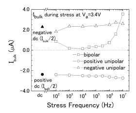
Fig. 3. Bulk current measured during stress as a function of frequency of the sample of Fig. 1. For comparison, the values of dc stresses were divided by two taking the 50% duty factor into account.  $I_{\rm bulk}$  was averaged from the  $I_{\rm bulk}$  values measured at the first 10 s stress.
